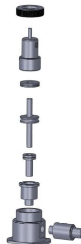
Fig 9-7. Disassembled FID collector
