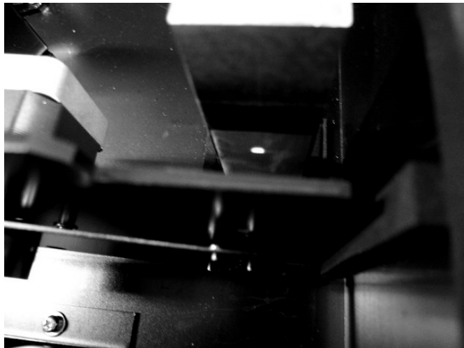
Adjustment of monochromator focus
