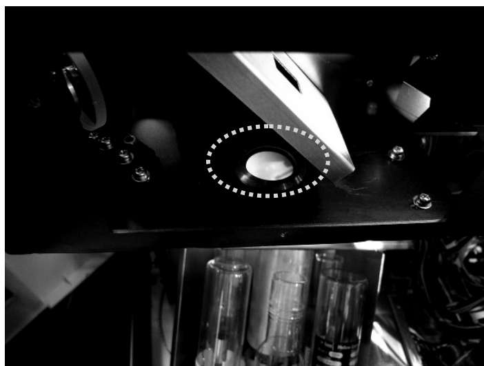
Installation of window plate assembly
